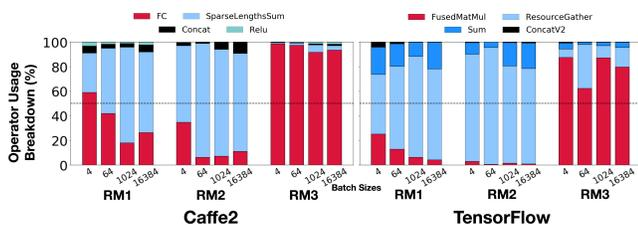
Fig. 7: **Comparison of Caffe2 and TensorFlow operator breakdowns** for DLRM-based recommendation models. Operators that comprise the majority of execution time are similar across both frameworks. Note, embedding table operations correspond to SparseLengthsSum in Caffe2 and the combination of ResourceGather and Sum in TensorFlow.
