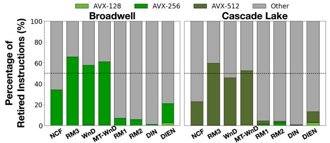
Fig. 9: **Instruction vectorization.** (Left) Broadwell AVX instructions constitute over 60% of retired instructions for models with larger FC layers (i.e., RM3, WnD, MT-WnD). (Right) Cascade Lake’s wider SIMD-width results in shorter execution time despite reduced AVX instruction footprint.
