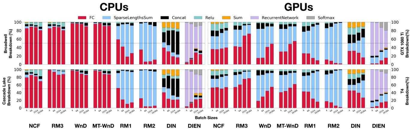
Fig. 6: **Caffe2 operator breakdowns** with CPUs (left) and GPUs (right). Models readily accelerated by GPUs are dominated by matrix operations (i.e., FC in red and recurrent layers in purple). Operator breakdowns between CPUs and GPUs vary significantly — models dominated by FC execution time on CPUs spend a large fraction of time on other operators on GPUs.
