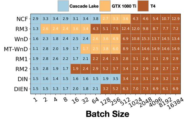
Fig. 5: Optimal hardware for each model architecture and batch size: each grid cell show the speedup over Broadwell when using the optimum hardware (color).
