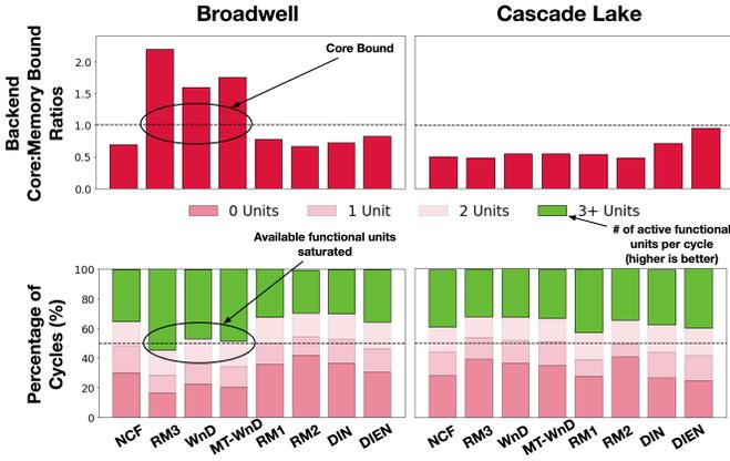
Fig. 10: **(Top) Ratio of Core:Memory Backend Bound cycles.** Majority of stalls come from functional units on Broadwell and from memory subsystem on Cascade Lake. **(Bottom) Functional unit usage.** RM3, WnD, and MT-WnD saturate Broadwell’s functional units more than other models with a large fraction of cycles that use 3+ units out of 8. Cascade Lake decreases the pressure on functional units.
