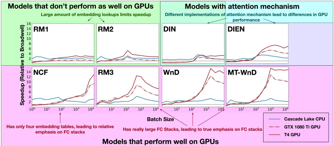
Fig. 3: **Systems performance evaluation** represented as speedup over Broadwell CPU across models, batch-sizes, and hardware platforms. Models are grouped into three primary, overlapping categories – ones that perform well on GPUs, ones that have comparable performance on CPUs and GPUs, and attention-based models with varying implementations.
