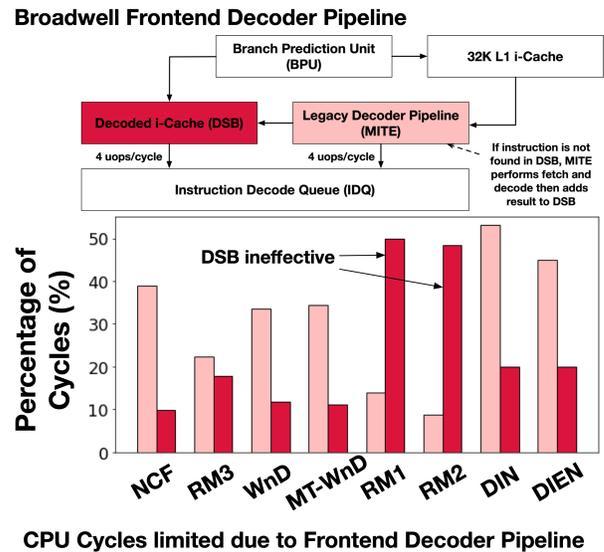
Fig. 13: **Frontend Decoder Pipeline Inefficiencies.** The two main decoder microarchitecture components are DSB and MITE. Shown are percent of cycles in which the CPU was limited by a specific decoder component (i.e., component was not supplying IDQ with optimal number of decoded instructions).
