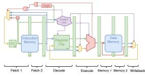
Figure 3: The original 7-stage pipeline RISC-V processor modified to XOR branch values with hash function outputs.
